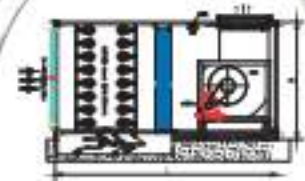
Air Scrubber Unit
